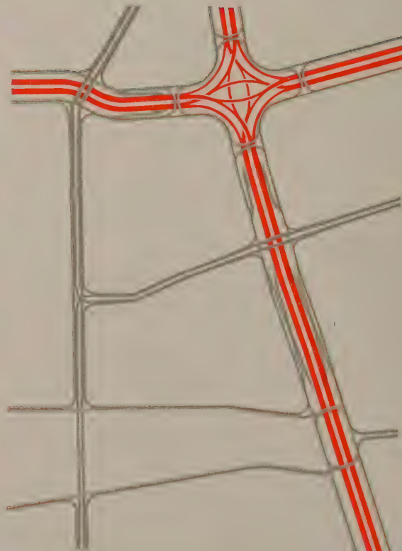
191 In order to reduce noise and severance the primary and district distributors are here combined.
